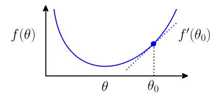
Derivative is slope of the function, so negative derivative points "downhill"
